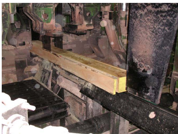
Figure 6. The McKee twin bandsaw at Auswest Timbers, Pemberton, equipped with chipper reducers (in this photograph hidden ahead of the saws) that effectively make four cuts on the initial pass. This photograph was taken during a trial back-sawing pruned 22-year-old plantation-grown E. globulus and shows the sawing immediately after the first turn-down
