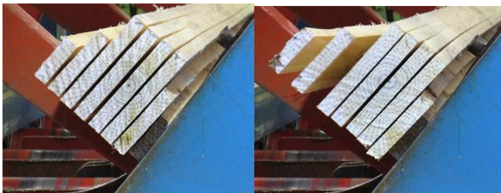
Figure 11. The approximate range in board deflection for 17-year-old E. nitens logs observed in trials with the HewSaw R250
