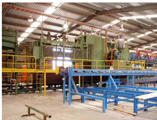
Figure 9. The HewSaw R250 at the Carter Holt Harvey Mill in Gippsland
