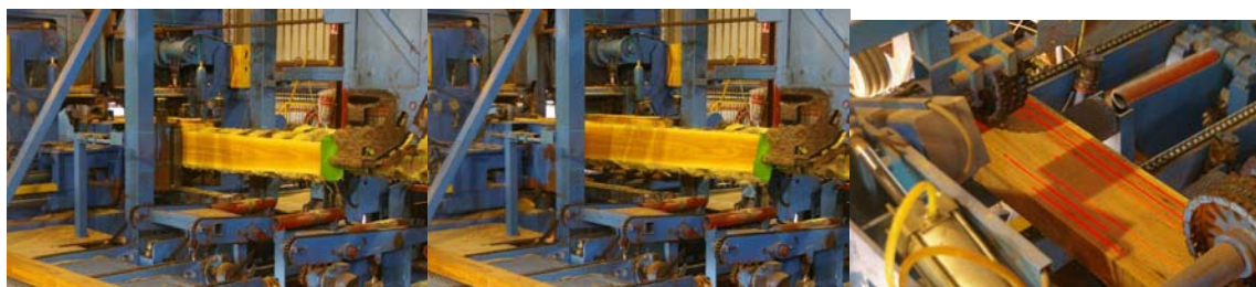
Figure 7. The system at Whittakers Timber Products processing 17-year-old pruned plantation-grown E. saligna . Left: sawing on the twin bandsaw; (centre) the hydraulic turn-down device in operation; (right) scanning of the central cant prior to sawing on the multi-saw
