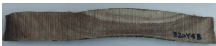
Figure 17. High shrinkage and cupping from damaging levels of tension wood in 22-year-old E. globulus (from Washusen et al. 2004)
