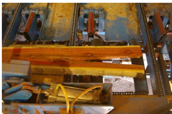
Figure 8. Log end-splitting in 17-year-old E. saligna , the consequence of sawing to produce a cant that is too thin relative to the log diameter
