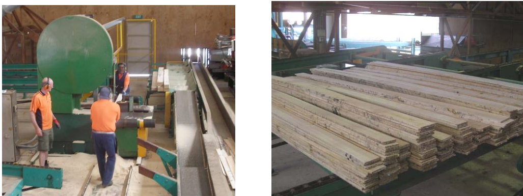
Figure 3. Resawing of flitches to produce 9mm-thick quarter-sawn boards
