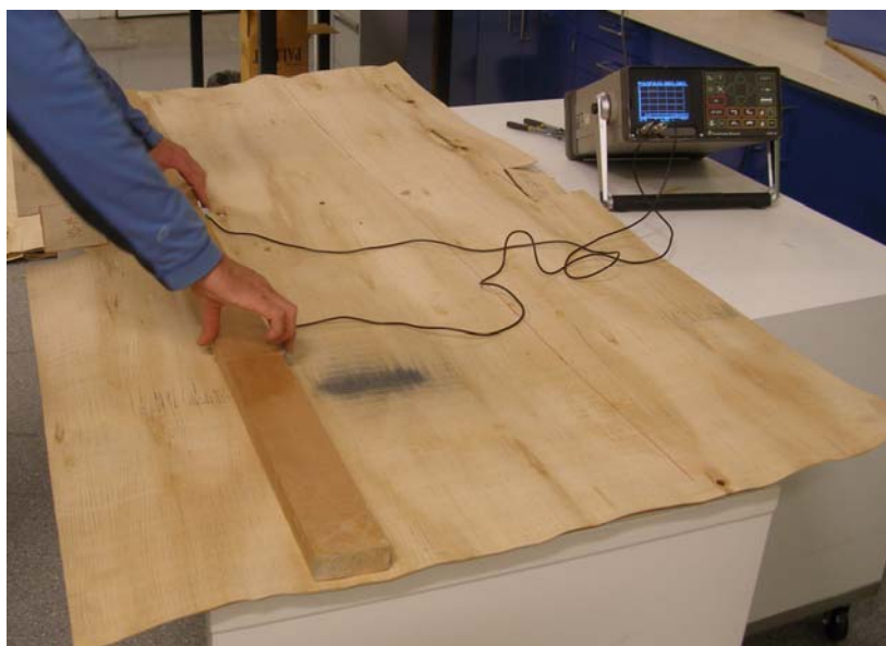
Figure 8. Measurement of acoustic wave velocity in longitudinal direction
