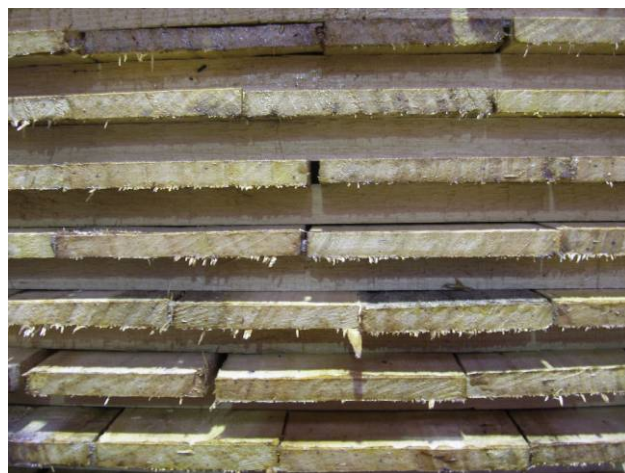
Figure 10. Board cross-sections after reconditioning
