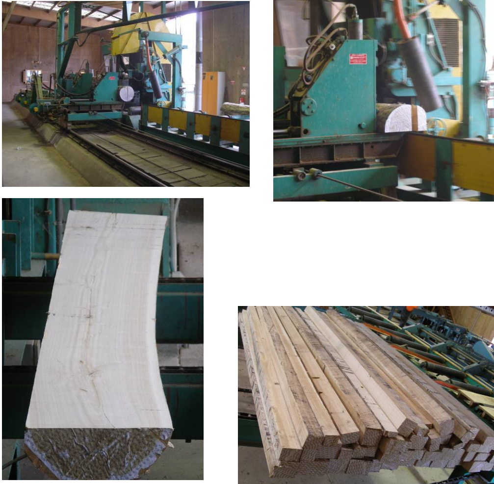
Figure 2. Sawing to produce flitches for re-sawing, at Creswick Timber Training Centre
