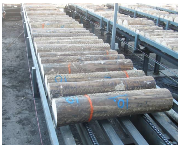
Figure 5. Billets on the in-feed conveyor line prior to veneering
