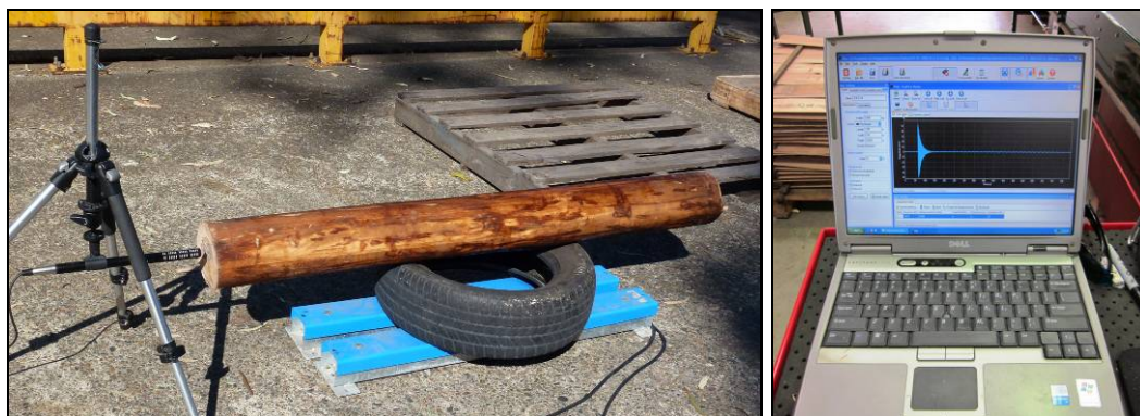
Figure 5. Acoustic testing of peeling billets to obtain dynamic MOE using Bing device
