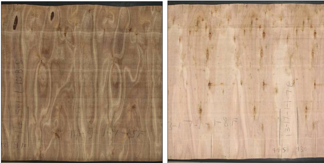
a) Figure 7. Examples of veneer sheet sample with labelling: a) CCV; b) E. dunnii
