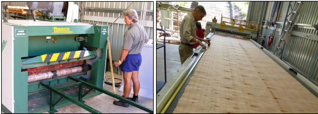
a) Figure 6. Processing of CCV billets into veneer sheet using an Omeco spindleless lathe b)
