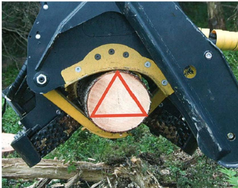
**Figure 3.** Cross-section of an eccentric stem being gripped at three points by a harvesting head (Uusitalo, 2010)
