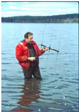
**Fig 4.** Radio tracking an implanted carp using a hand held yagi
