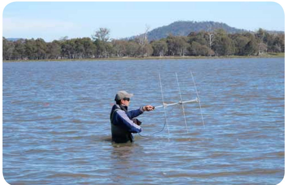
Figure 12. A member of the carp team using a handheld aerial and lotek receiver to pin-point the position of a transmitter fish.
