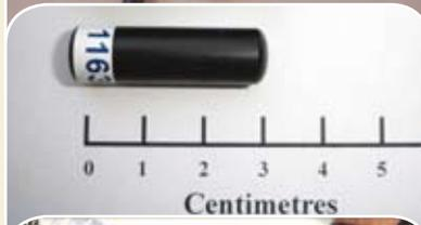
Acoustic tag used for tracking fish movement (photo courtesy of TAFI).
